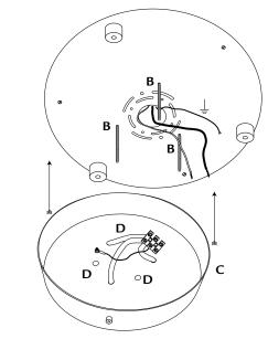
4. Secure the cover against the fixture **A** screwing the 3 screws E on the 3 nipples **B**.
